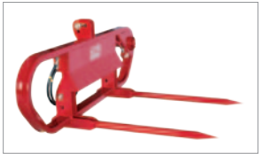
2-1/4 inch high tensile tapered fork tines are used to load bales. One tine is longer to simplify reattachment to the feeding cradle.
