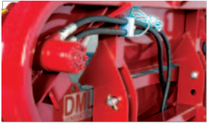
The hydraulic motor is mounted out of harm's way inside the headstock frame.
