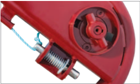
The spring loaded locking pin latches the headstock to the feeding cradle, and its position close to the motor guarantees the Tee drive stays engaged during operation.
