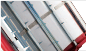
6mm zinc plated steel bars have aggressive tapered teeth to tear and release feed material freely.
