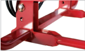
The linkage plates, not the tines, carry the weight of the feeder. There are 2 linkage pin heights and the pin position carries the feeder close to the back of the tractor.
